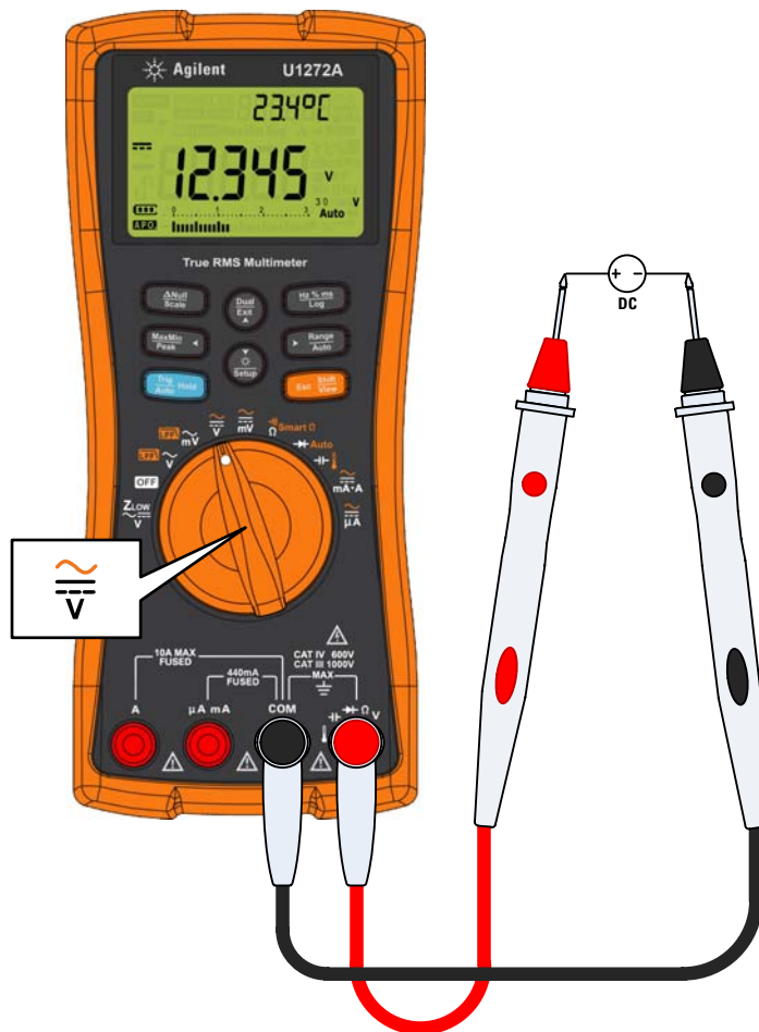
Figure 2-6 Measuring dc voltage
