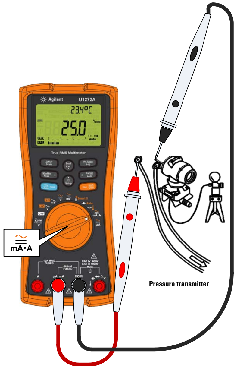
Figure 2-34 Measuring dc current using the 4-20 mA % scale
