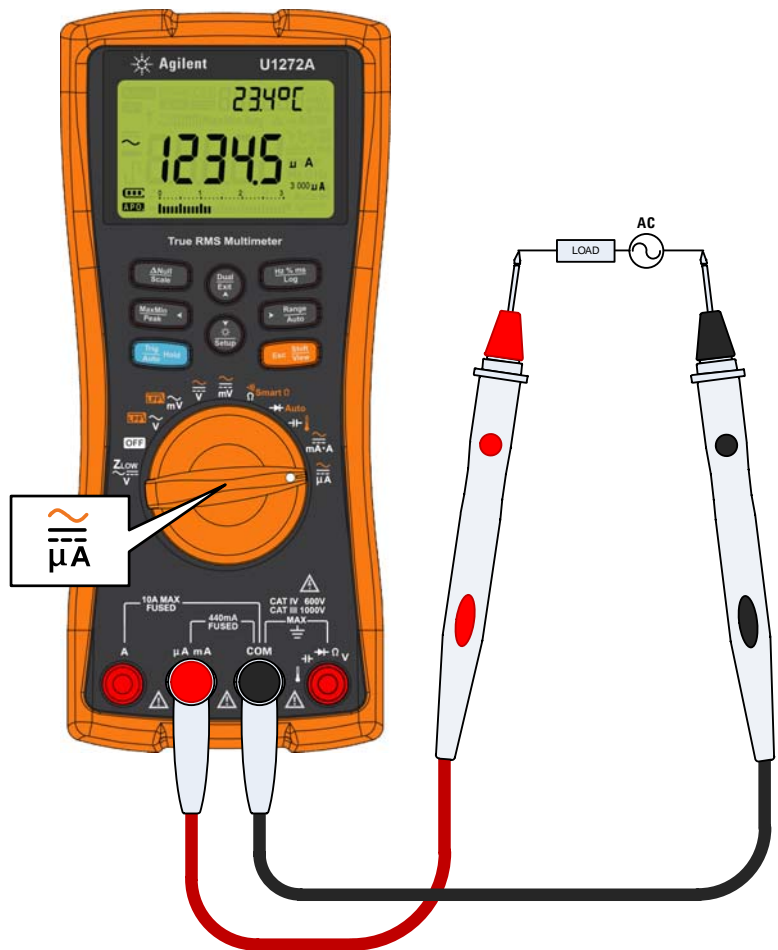
Figure 2-31 Measuring ac current
