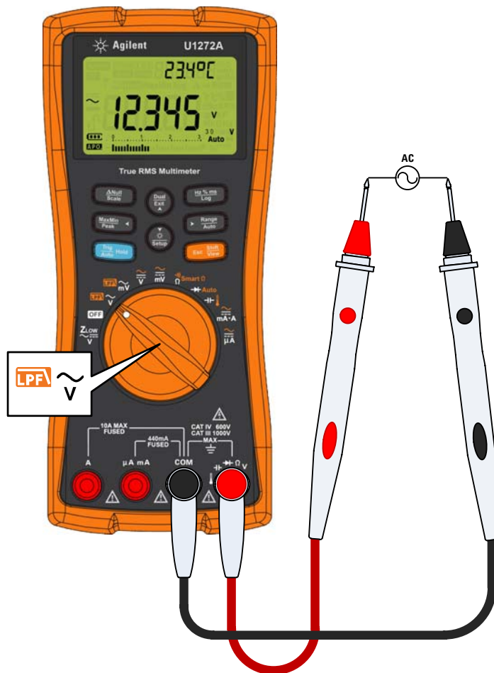
Figure 2-2 Measuring ac voltage
