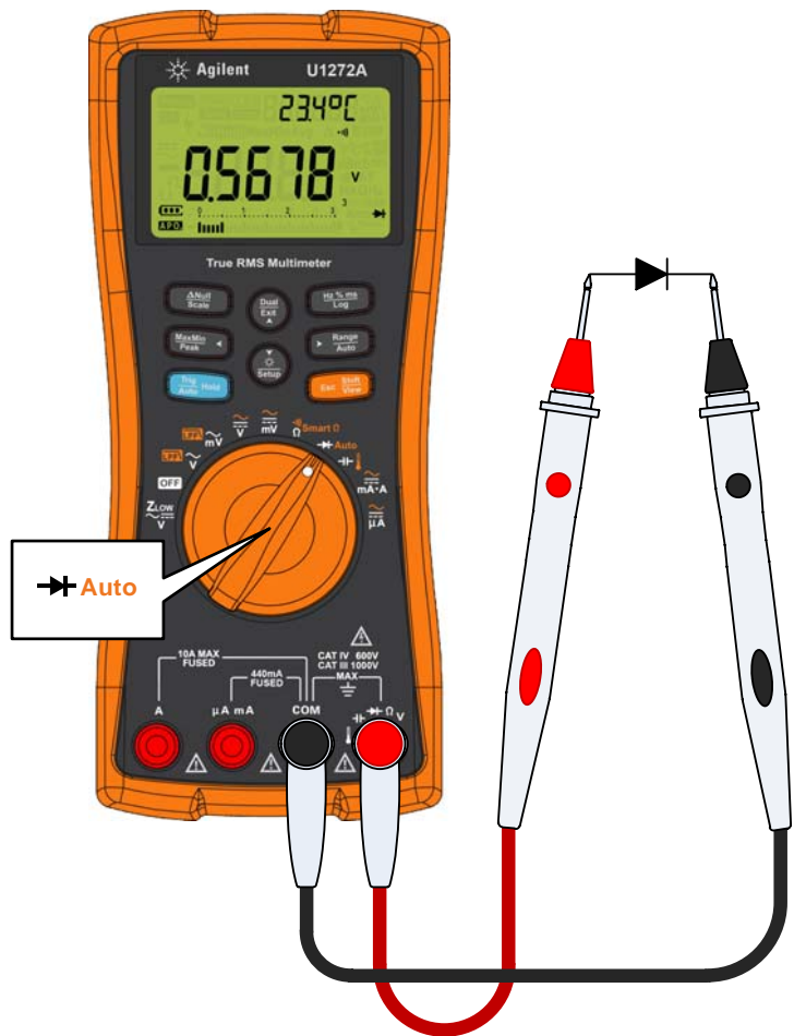
Figure 2-20 Testing forward bias diode
