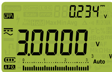
Figure 2-4 DC coupling for ac+dc voltage measurements
