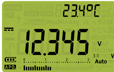
Figure 2-5 DC voltage display
